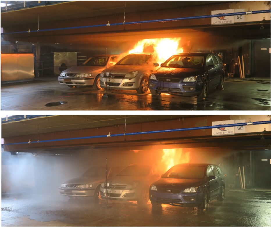
Figure 6. Test 2: The fire size at 02:49 [mins:], moments before water was discharged through the six automatic sprinklers that had activated (top) and two minutes thereafter (bottom) at 04:49 [mins:].
