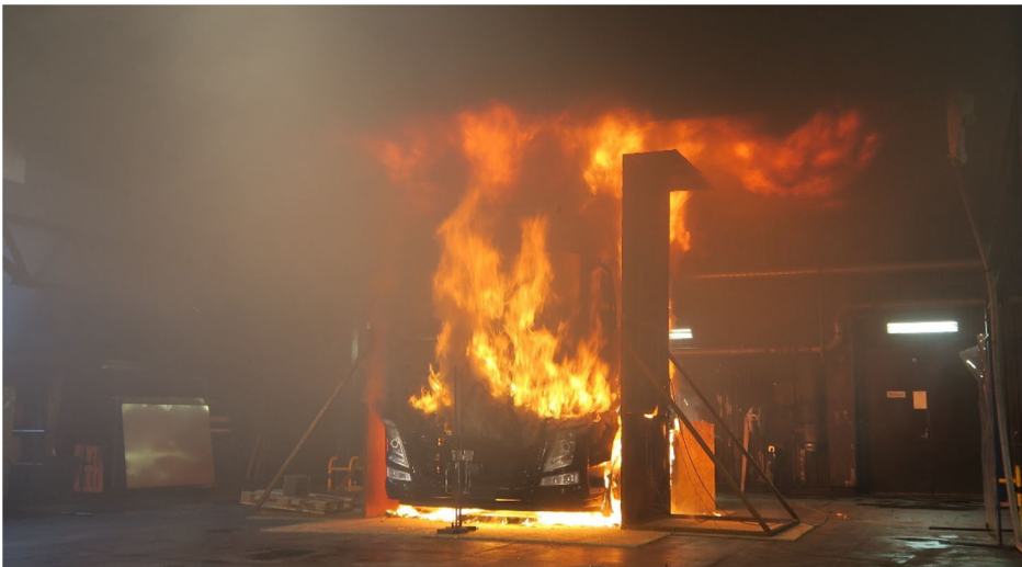
Figure 15. Test 6: The fire size at 02:00 [min:s], a few seconds prior to discharge of water from the sprinklers that had activated. Full discharge from the opened sprinklers was recorded at about 02:29 [min:s].
