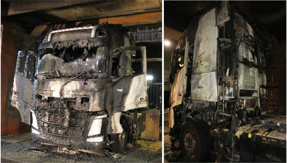
Figure 16. Test 6: External fire damage to the freight truck.
