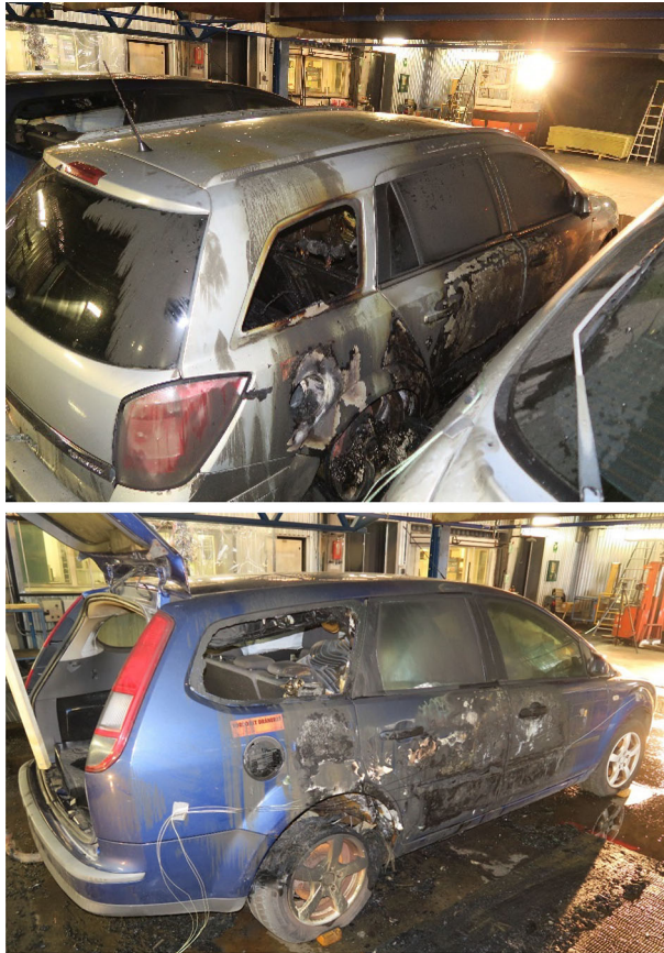
Figure 7. Test 2: The fire damage to the car in the middle (top) and to the car to the left (bottom) that was partly involved in the fire.
