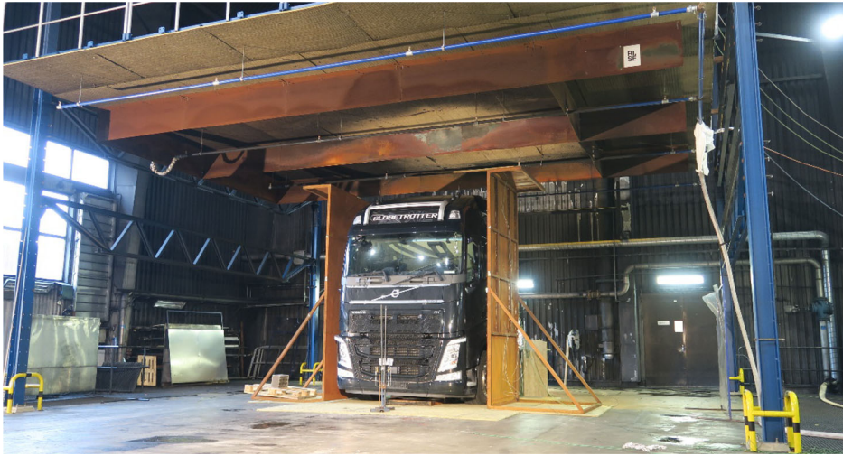
Figure 5. Test 6: The test set-up as seen prior to Test 6. The clear height, as measured from the floor to the underside of the ceiling beams, was 4.6 m.
