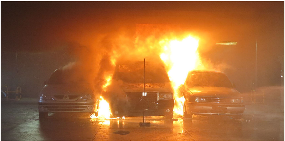
Figure 13. Test 5: Manual fire-fighting at 05:49 [min:s] using hose streams.
