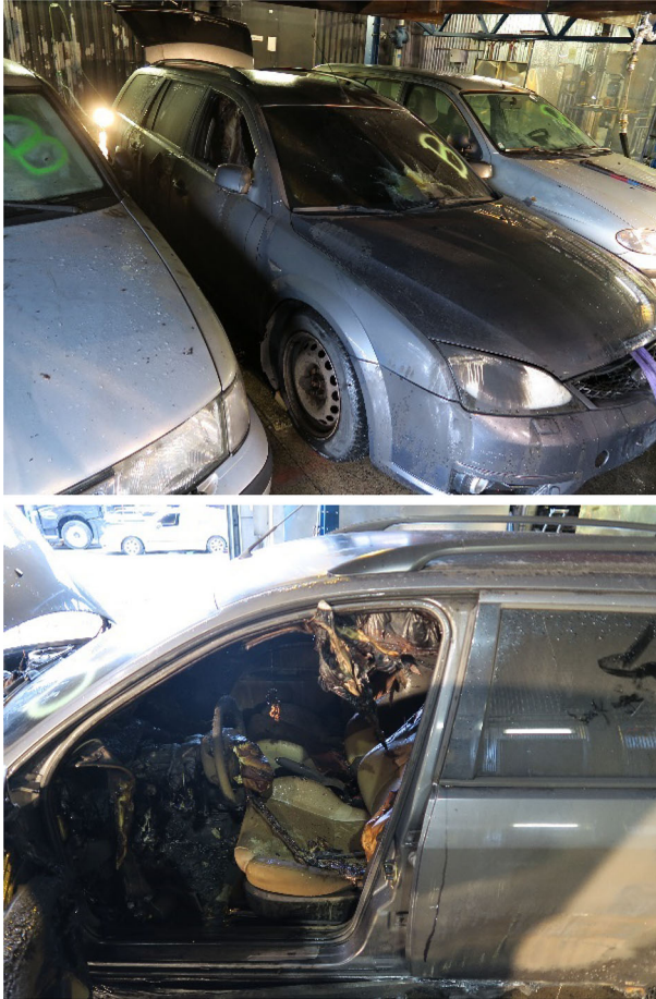
Figure 9. Test 4: The fire damage to exterior (top) and parts of the interior (bottom) of the middle car.
