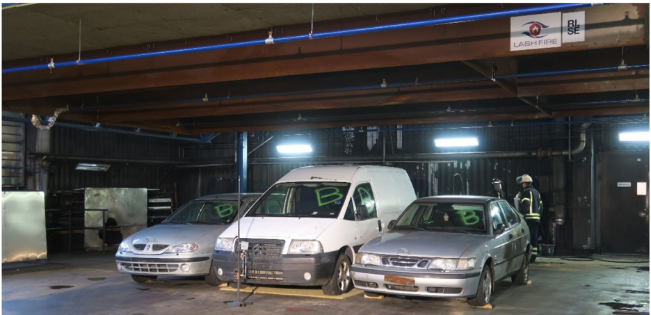
Figure 4. Test 5: The test set-up as seen prior to Test 5. The clear height, as measured from the floor to the underside of the ceiling beams, was 2.8 m.
