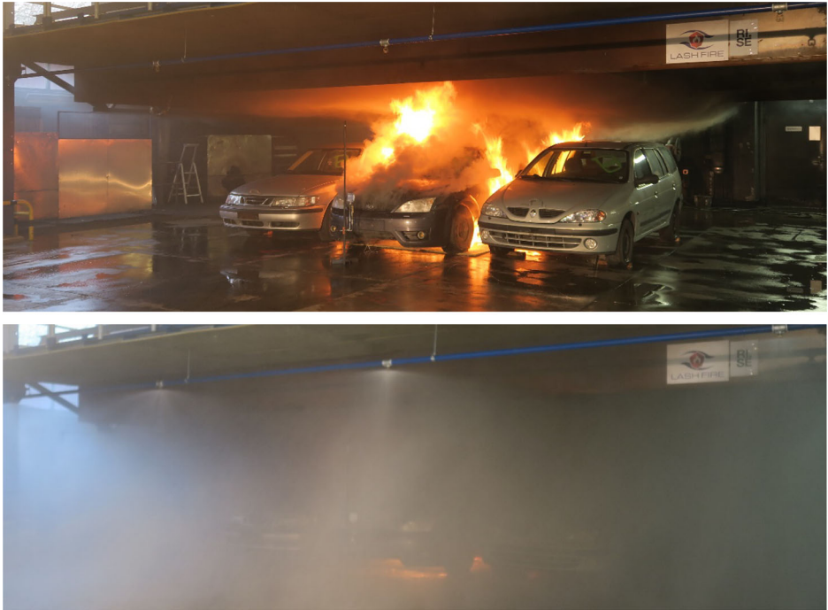
Figure 8. Test 4: The fire size at 04:00 [mins] (top) moments before and at 04:30 [mins] (bottom), shortly after the discharge of water of the deluge water spray system.
