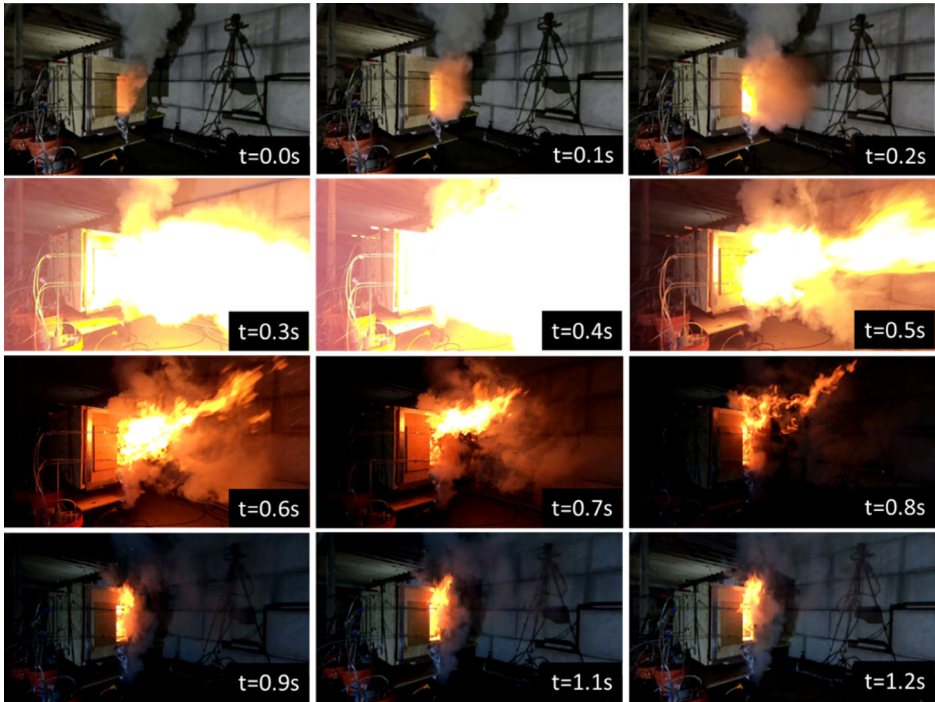
Figure 4. Sequence of video images 0.1 s apart, showing the external horizontal flame projection from an overpressure event from a 0.15 m wide by 0.4 m high vent opening. For scaling the images, the distance from the vent to the edge of the frame is approximately 2.5 m.
