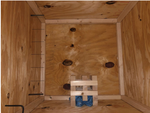
Figure 1. Photograph of the plywood compartment interior showing mineral spirits soaked paper towels below the crib just prior to ignition. For scaling the image, the rear wall of the compartment was 0.76 m high and 0.76 m wide.
