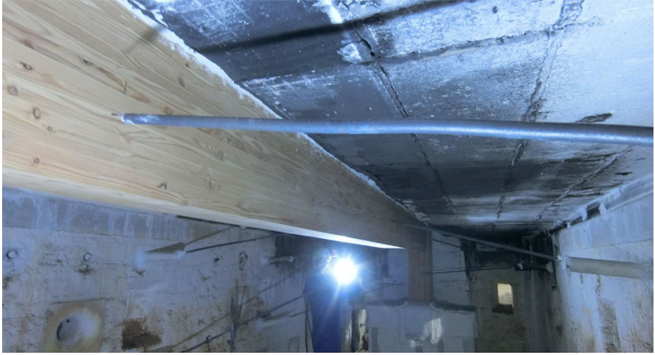
Figure 19. Specimen set in the furnace.
