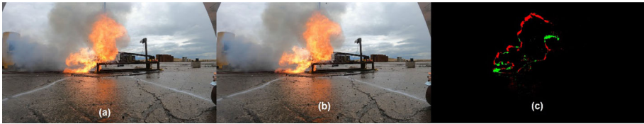
Figure 12. (a) camera ‘x’ during thermal runaway; (b) camera ‘x’ during thermal runaway, 1 frame (16.7 ms) after (a); (c) difference between (a) and (b).
