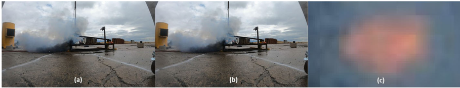
Figure 11. (a) camera ‘x’ before ignition; (b) camera ‘x’ at ignition, 1 frame (16.7 ms) after (a); (c) zoomed in version of (b) where ignition commenced.
