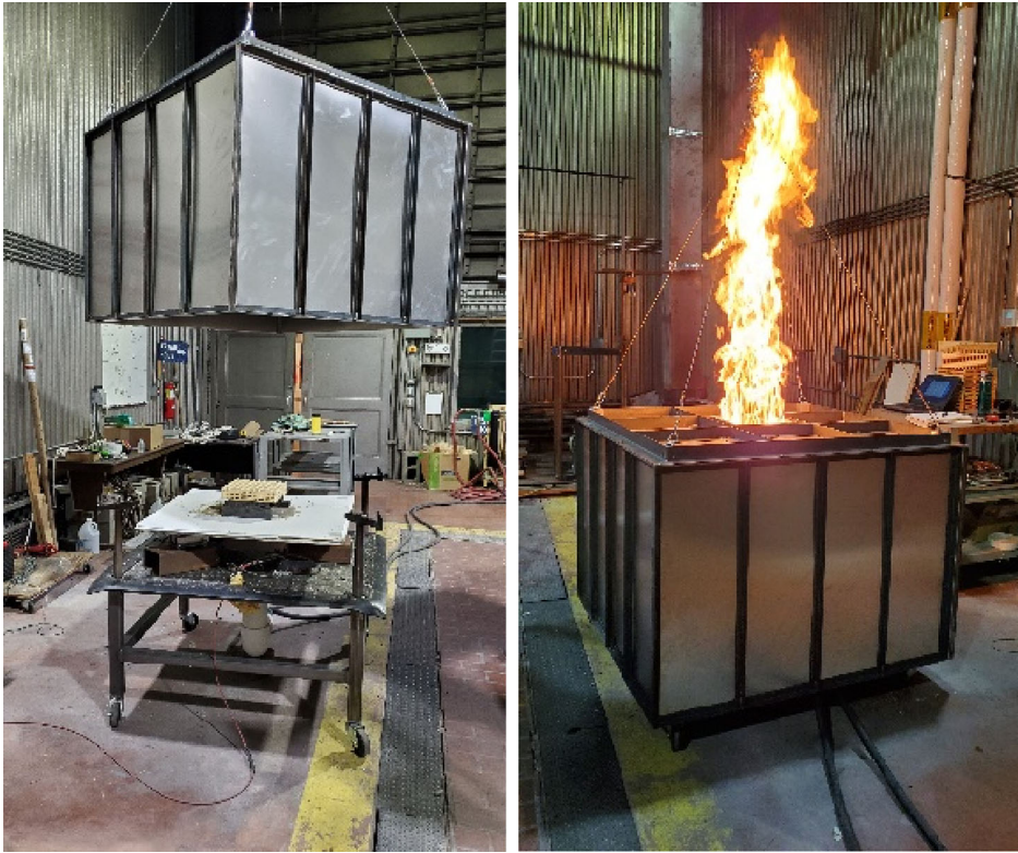
Figure 2. Left: Air box with lid up. Air enters the box through via PVC piping underneath the table. A rubber gasket prevents air from escaping downward from the box. Also seen are four adjustable supports that control the height of the lid. The weighing platform is covered in white ceramic paper insulation and sits on three (silver) load cells (one visible). Right: The lid is adjusted so that the top of the crib sits flush with the ventilation hole, ensuring that the airflow passes through the crib.
