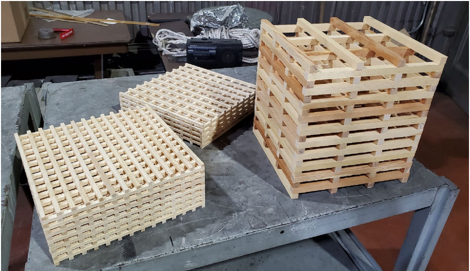
Figure 1. Example cribs. From left to right: densely-packed crib (crib design #9), transition (crib design #8), and loosely-packed crib (crib design #3).
