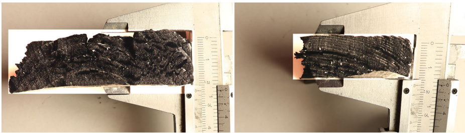
Figure 22. Charred specimens of spruce (left) and pine (right) after cone calorimeter testing in nitrogen, opened. The grain direction is towards the reader. The image brightness is adjusted in the specimen region to better reveal the char structure.
