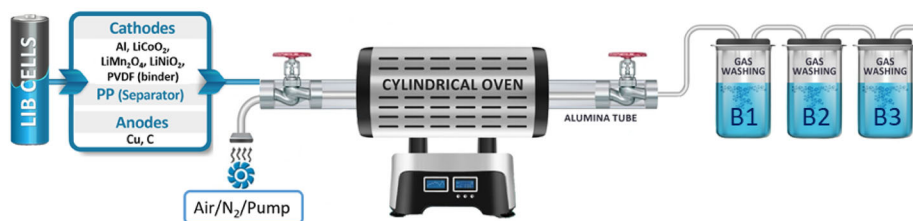
Figure 1. Apparatus with the washing system used for the simulation of the thermal accident.
