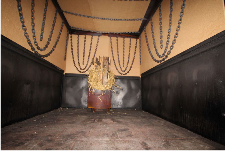
Figure 8. Example of low density wood fiberboard fuel load in the Fire Behavior Lab.
