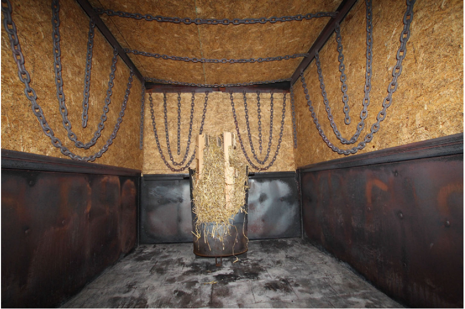
Figure 3. Example of an OSB fuel load in the Fire Behavior Lab prior to ignition.
