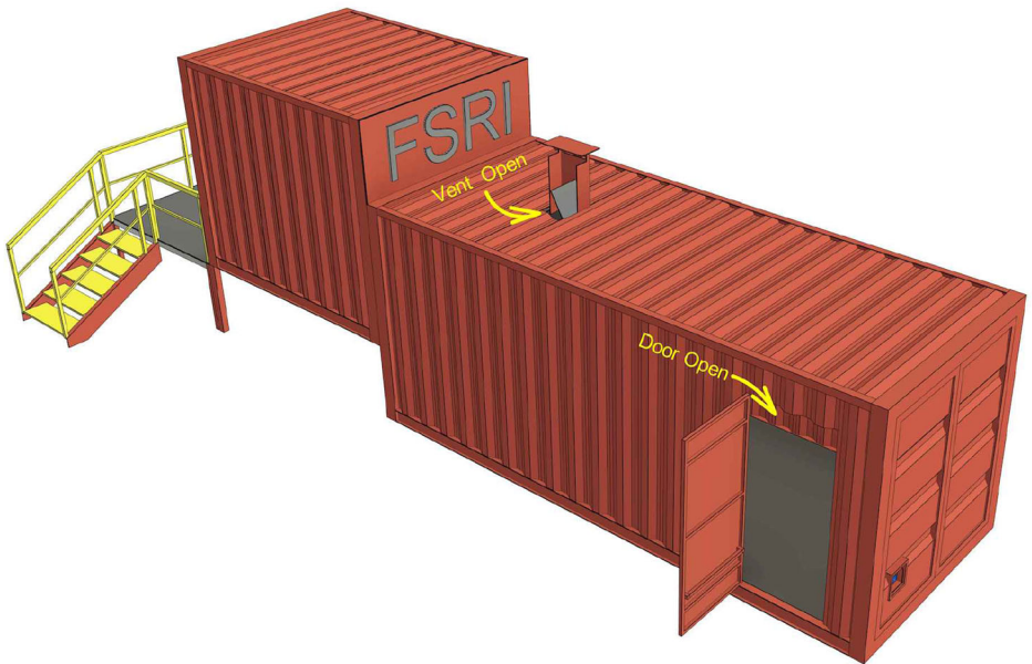
Figure 13. Pre-flashover vent position in the Fire Behavior Lab.
