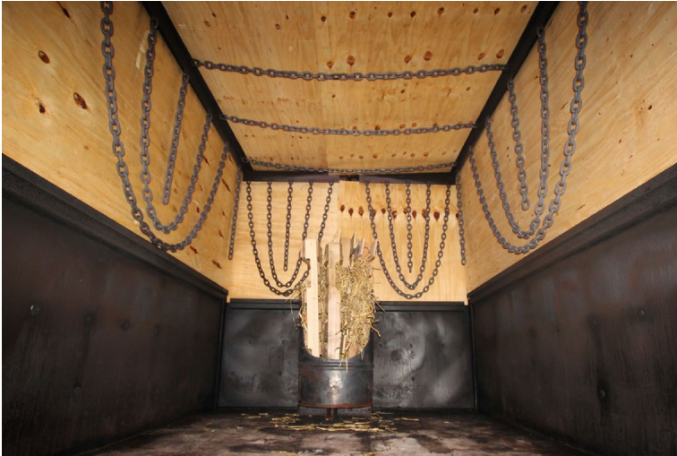
Figure 11. Example of plywood fuel load in the Fire Behavior Lab.
