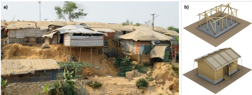
Figure 3. (a) Camp 8W 2 weeks before the fire [46]. (b) Standard shelter for fire response showing the bamboo frame and structure clad [14].
