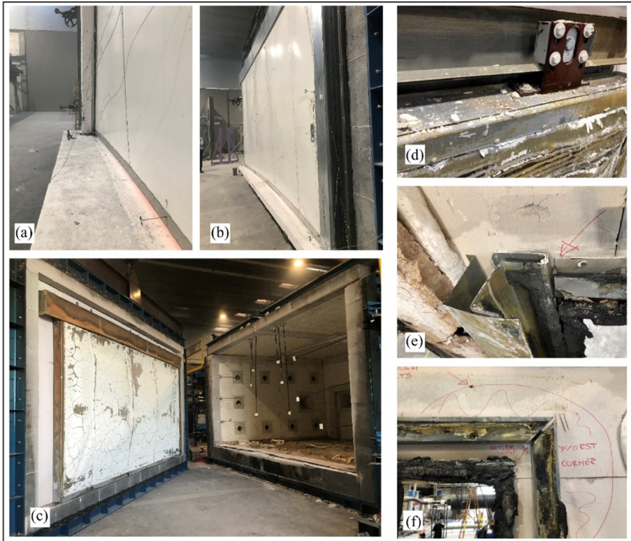
Figure 13. Post-fire views of sliding door tests.
