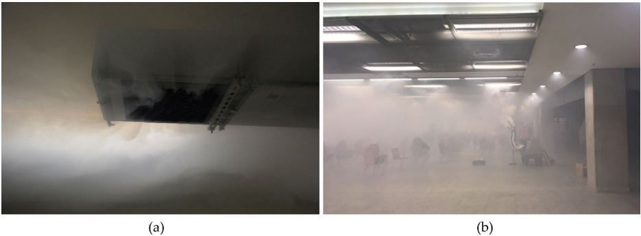
Figure 2. (a) The phenomenon of plugholing—cold air is removed through an exhaust point from below the layer of hot smoke; (b) disturbed smoke layer—no sharp layer interface visible anymore, smoke present in the whole height of the compartment.
