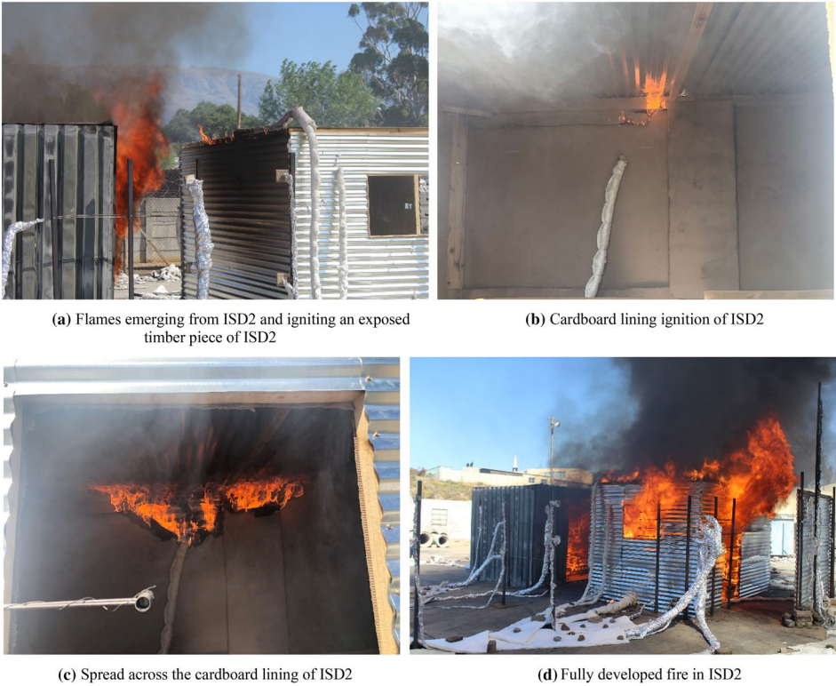
Figure 15. a Flames emerging from ISD2 and igniting an exposed timber piece of ISD2, b Cardboard lining ignition of ISD2, c Spread across the cardboard lining of ISD2, d Fully developed fire in ISD2.
