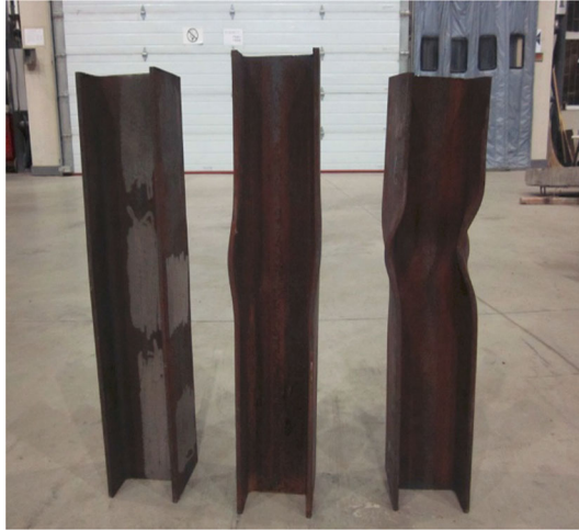
Figure 8. Buckling deformation at temperatures of 400°C to 600°C.
