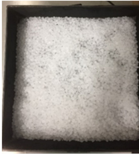
Figure 3. The PP fuel pellets in the fuel tray. The tray is 20 × 20 cm, the pellets are nominally 3 mm spheres.
