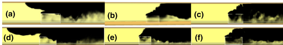
Figure 3. The effect of different velocities on smoke propagation of 10 MW and 30 MW vehicle fires in the road tunnel at t = 100 s (a) 10 MW, 1.5 m/s, (b) 10 MW, 2.8 m/s, (c) 10 MW, 5 m/s, (d) 30 MW, 1.5 m/s, (e) 30 MW, 3.7 m/s, (f) 30 MW, 5 m/s.
