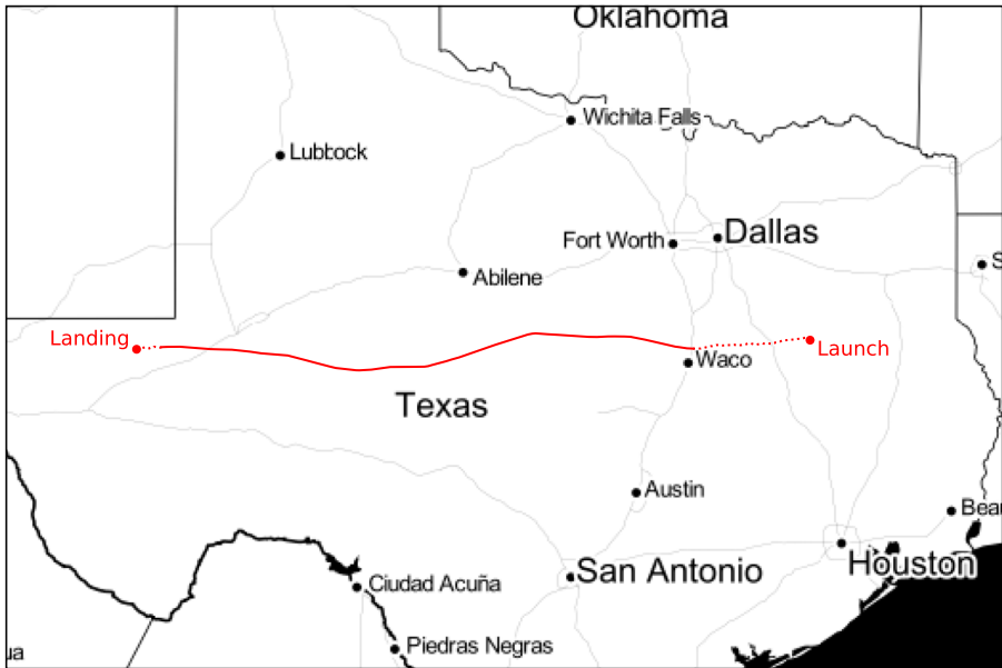
Fig. 6 Map of the balloon flight path. The solid red section indicates where the balloon was at the float altitude of 37.4 km. The dotted sections indicate the ascent and descent phases of the flight
