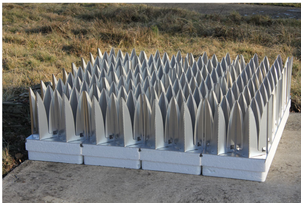
Fig. 2 The Vivaldi antenna array tile for SKA MFAA, developed in ASTRON, The Netherlands
