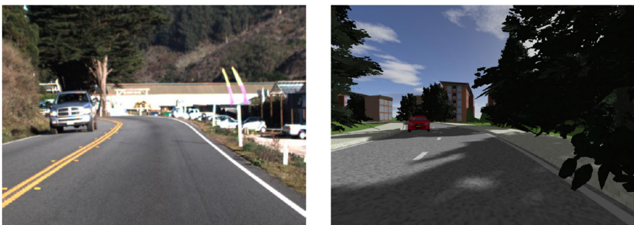
Fig. 3 Example of simulator-generated driving image from PreScan corresponding to a real-world image (Haq et al. 2020)
