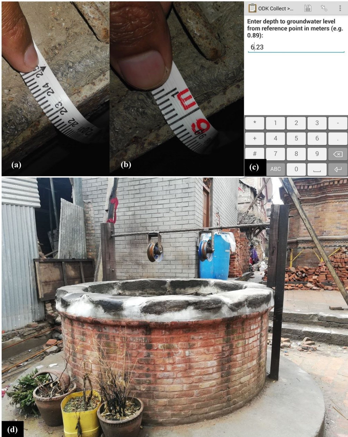
Fig. 3 a Image of the measuring tape and reference point when the measuring tape just touches the groundwater surface. b Image of the measuring tape and reference point when the measuring tape is pulled up so that the next whole meter on the
