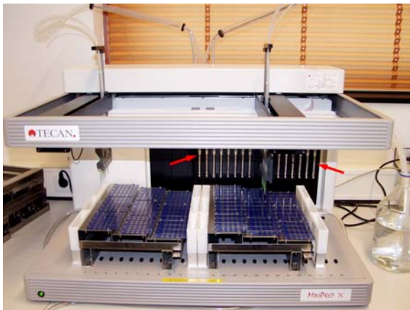
Fig. 2 Tecan Miniprep 75/2 robotic sample processor, showing two work areas with 36 IF slides each and two robotic arms with 8 pipette tips each (red arrows)
