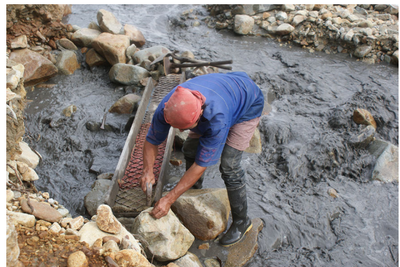
Fig. 4 A barequero working a sluice box in Qda. Cascabel at its confluence with the Rio Cauca. Note the high quantities of sediment in the creek from slurry discharged from the entables
