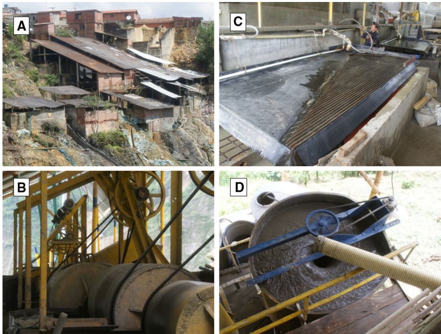
Fig. 2 a Gold ore processing in an entable in Marmato. b Ore is first crushed by jaw crusher and then (b) ground in small ball mills called cocos . c Gold and auriferous pyrite are separated by
