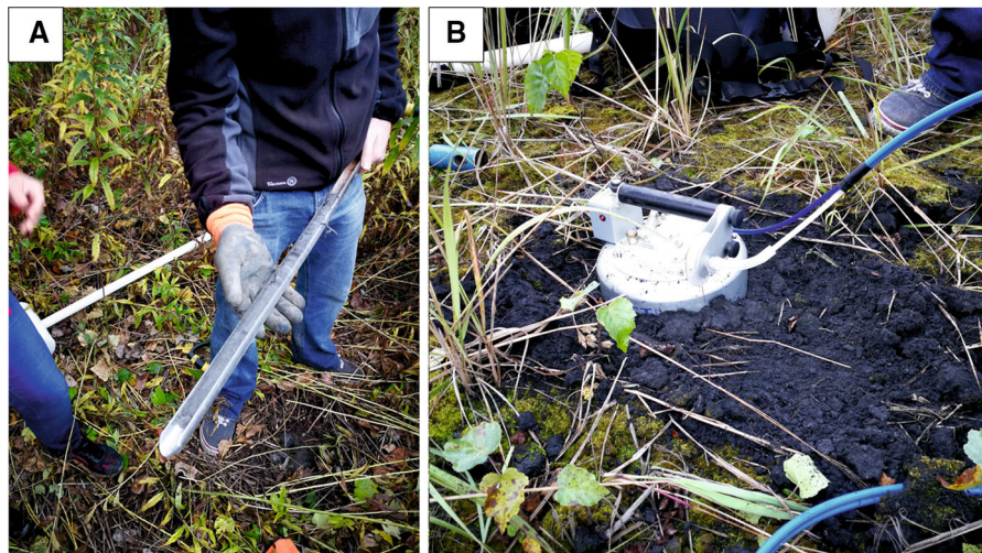
Fig. 2 Collection of soil samples using the Egner's stick (a) and measurement of gases emission using static chamber method (b)
