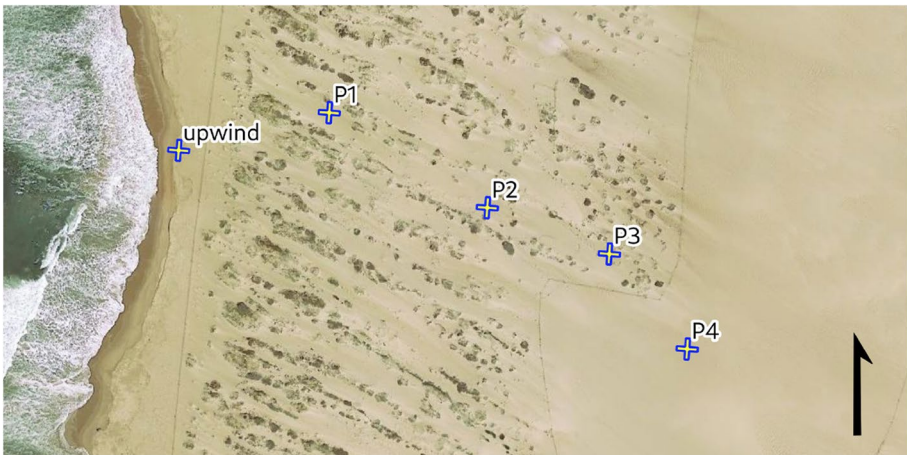
Fig. 5 Monitoring locations for the sonic anemometers. Sites P1–P4 were visited by one mobile tower, while another was held fixed at the upwind location
