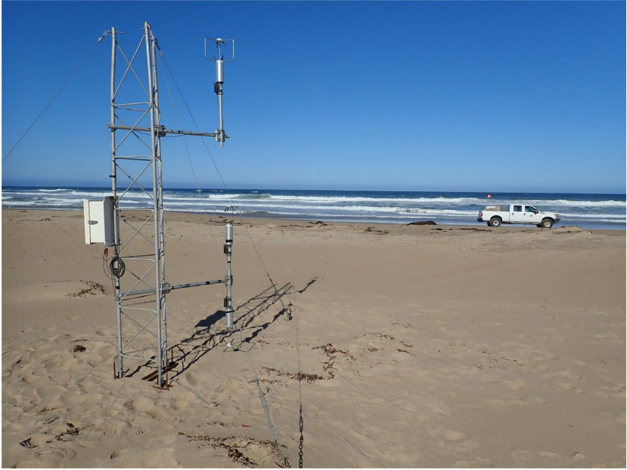
Fig. 4 Tower configuration for data collected with the sonic anemometers
