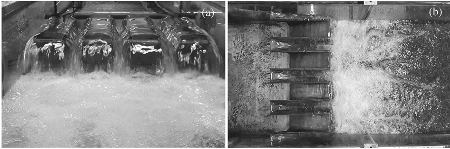
Fig. 3 Pictures of the PK weir: a frontal view; b plan view (flow from left to right)
