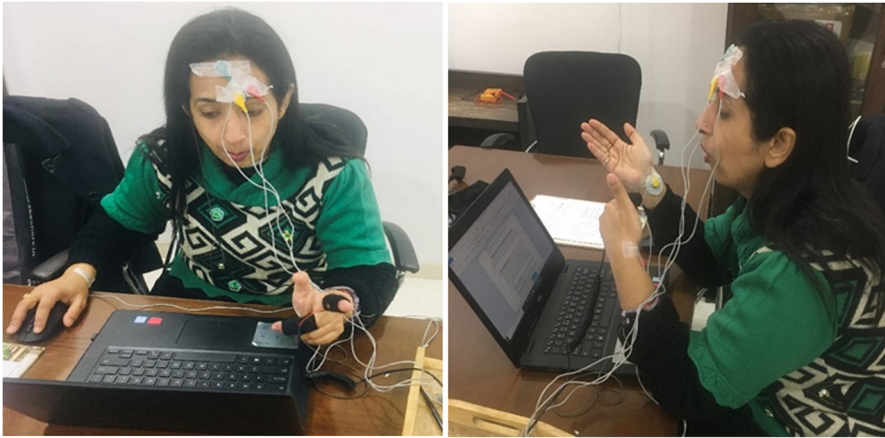
Fig. 4 Subject taking an online class by wearing three sensors: ECG (wrist), GSR (fingers), and fEMG (eyebrows)
