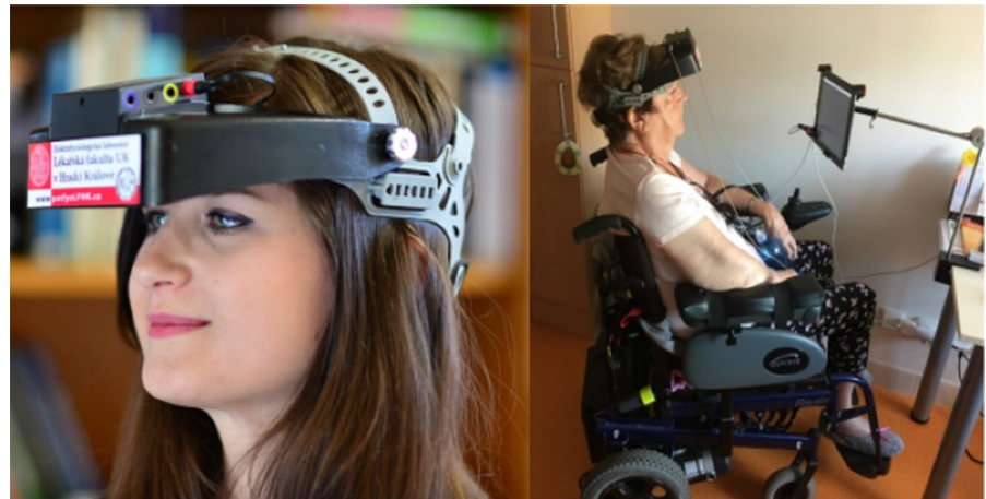
Fig. 2 Arrangement of VEP examination with the built-in LED stimulator (left) and in an immobilized patient (right) with the use of the external stimulator in the adjustable holder
