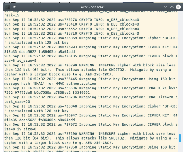
Fig. 6 Output delivered by the server to the openvpn command when used with the -secret and increased verbosity
