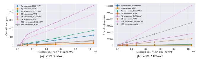
Fig. 4 Benchmarking of the MPI Reduce and AlltoAll Collective routines
