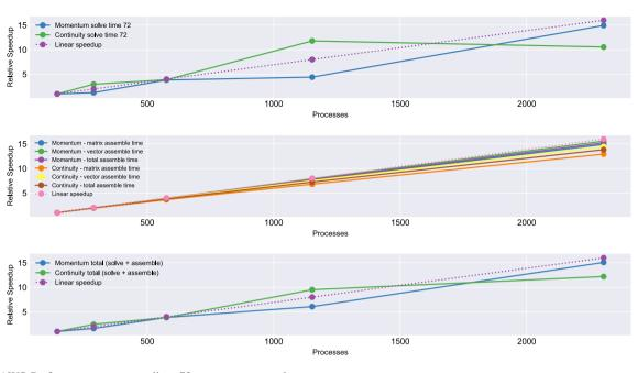
Fig. 12 AWS Performance, strong scaling, 72 processes per node
