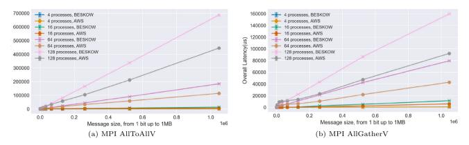
Fig. 5 Benchmarking of the MPI Alltoallv and Allgatherv Collective routines
