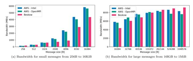
Fig. 2 Bandwidth between 2 nodes on AWS with Intel and Open MPI, and on Beskow with Cray MPI
