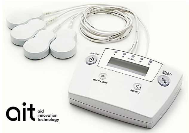
Fig. 1 ait® (AT-04), a minimally invasive device developed by Peace of Mind Co., Ltd., that consists of a controller and dual-coil emitter assembly, irradiating a mixed alternating magnetic fields
