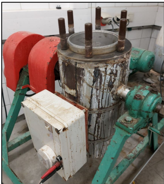
Fig. 4 Rotary digester used for the experiments. The reactor lid is not present in the picture
