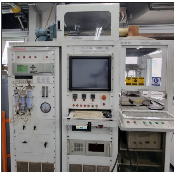
Fig. 3 International Organization for Standardization 5660–1 (Cone calorimeter)
