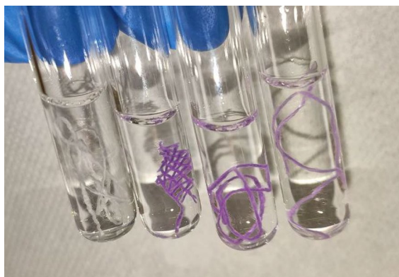
Fig. 2 From the left, Schiff test on G-cotton, oxidized G-cotton from the 1st use of the oxidation solution, oxidized G-cotton from the 2nd use of the oxidation solution, oxidized G-cotton from the 3rd use of the oxidation solution
