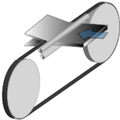
Fig. 4 Illustration of the splitting process using a Fortuna Splitting Machine
