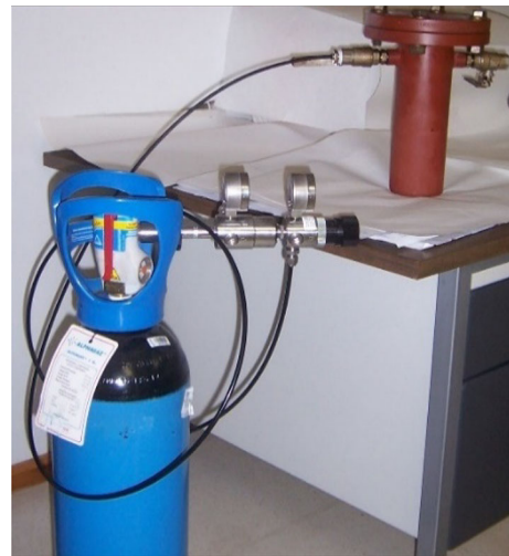
Fig. 1 Vessel for thermal ageing
