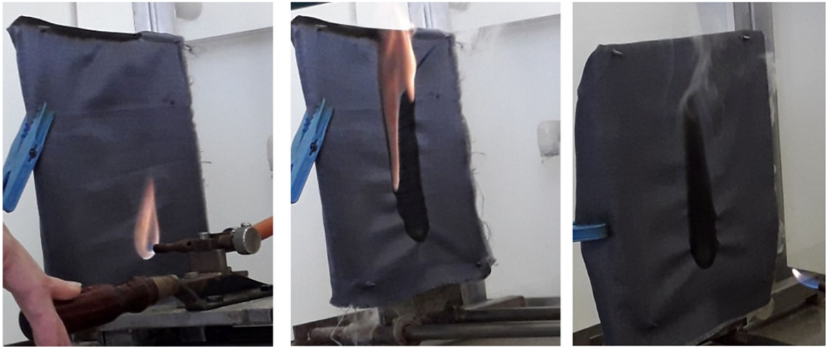
Fig. 8 Flammability testing of 1.5MFC-AP printed fabric in compliance with EN ISO 15,025
