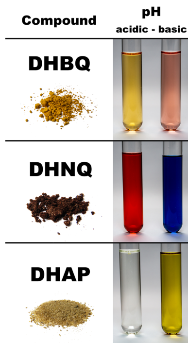
Fig. 1 The three cellulosic key chromophores DHBQ (1), DHNQ (2), and DHAP (3) as neat solids and in acidic and alkaline aqueous solution (approx. 1 mM)
