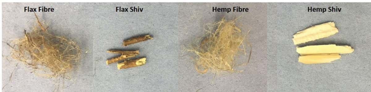
Fig. 1 Optical photos showing the appearance of studied fibre and shiv of flax and hemp
