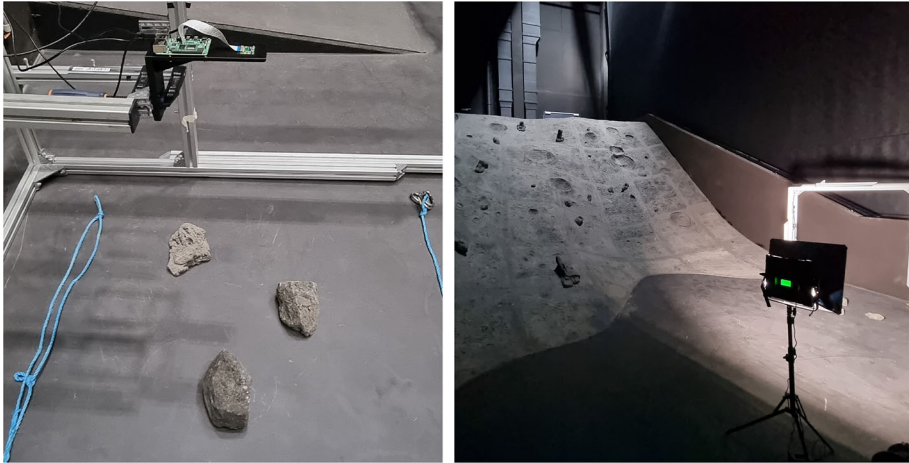
Fig. 22 Set-up used at DFKI Bremen for the image acquisition. On the left, a close-up look on the mount used to hold together the camera and the processing unit. On the right, an overview of the Space Hall before completely darkening the room
