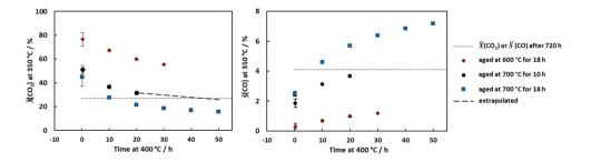
**Fig. 9** Mean conversions  $\overline{X}(CO_2)$  (left) and mean selectivities  $\overline{S}(CO)$  (right) of chosen aged Ni/ $\gamma$ -Al<sub>2</sub>O<sub>3</sub> catalysts of the reference measurements at 350 °C over 6 h in dependence of the reaction time of the catalyst at 400 °C. The indication bar indicates the decrease of  $\overline{X}(CO_2)$  and the increase of  $\overline{S}(CO)$  at 350 °C. The dotted horizontal
