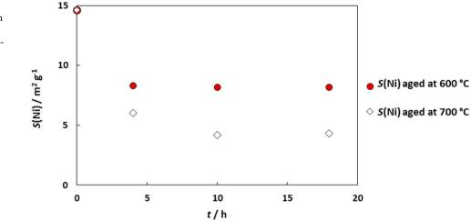
The Ni surface area is determined with  $H_2$  chemisorption. Figure 6 shows that the metal surface decreases strongly within the first 4 h of the aging. Stabilization of the surface is achieved after 4 h (600 °C) and after 10 h (700 °C). After aging at 700 °C, the metal surface decreases more strongly than after aging at 600 °C. It is also noticeable that the decrease of the metal surface is more significant than the decrease of the BET surface.
