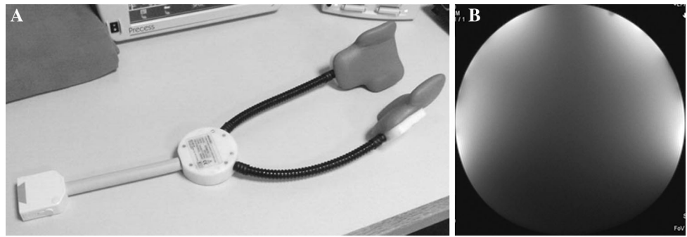
Fig. 1 Dedicated surface coils provide improved signal-to-noise ratio for superficial structures (a). When these coils are applied to a cylindrical water phantom, measuring 6 cm in diameter, the drop-off in signal intensity on the T1-weighted images provides a visual demonstration of the penetration depth of the coil (b)
