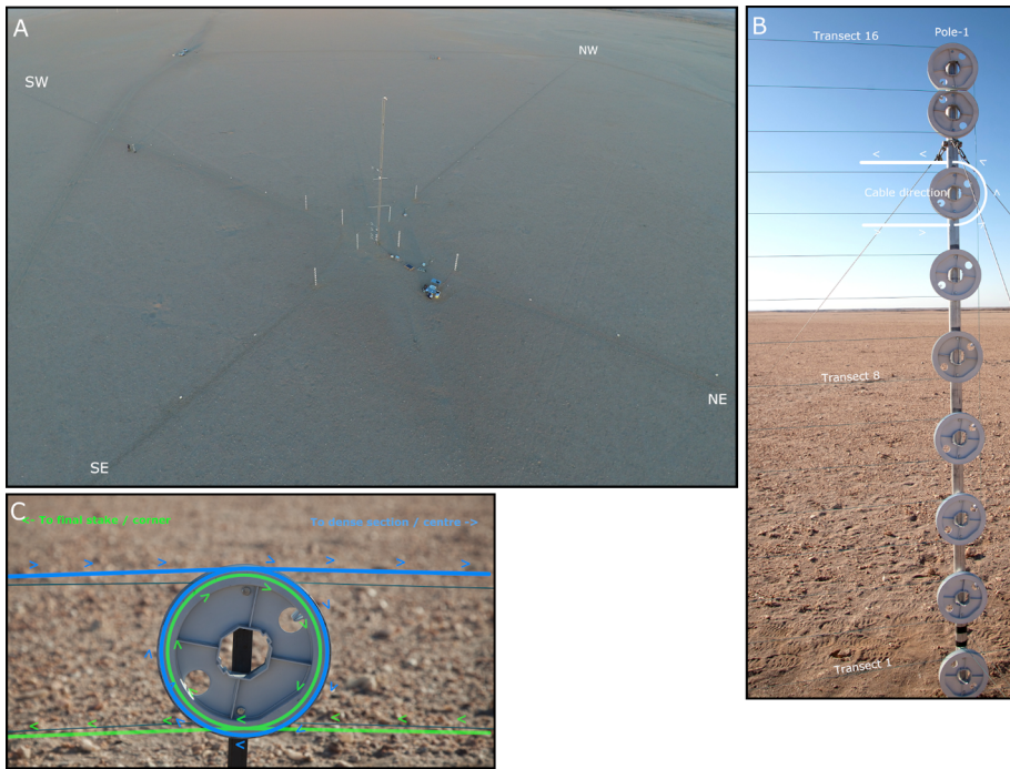
Fig. 1 Photos from the NamTEX field site. A Aerial view showing central mast and X footprint of the DTS system. B One of the dense section poles showing 16 dense transect heights and the cable routing. C One of the long section stakes showing cable routing around the support disk
