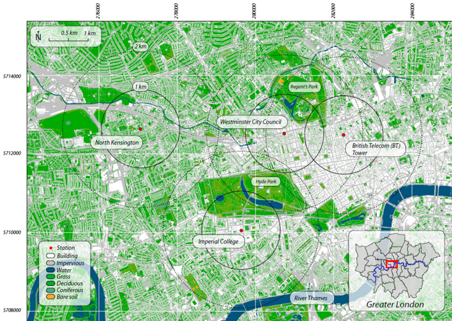
Fig. 1 Land cover map (based on OS MasterMap) of Central London with locations where instrumentation was placed: North Kensington, Imperial College, British Telecom (BT) Tower and Westminster City Council (WCC). Map of the Greater London Area is shown in the right inset. Rings are radii of 1 km from measurement locations. The grid is labelled as metres (easting, northing), UTM zone 31N
