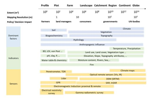
Fig. 1 Mapping and monitoring peatland status and conditions across scales. BD bulk density, LOI loss of ignition, TDR time domain reflectometer, Vis visible wavelength, IR infrared, LiDAR light detection and ranging, DEM digital elevation
