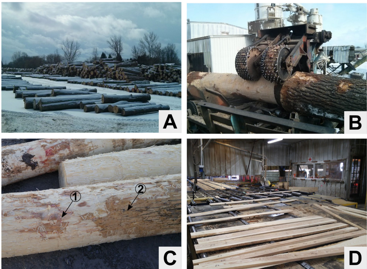
Fig. 3 In the sawn wood production process, round wood (A) is first mechanically debarked, using machinery such as a rotary-head debarker (B). Debarked wood (C) may show evidence of insect damage (arrow 1) and can still retain some
