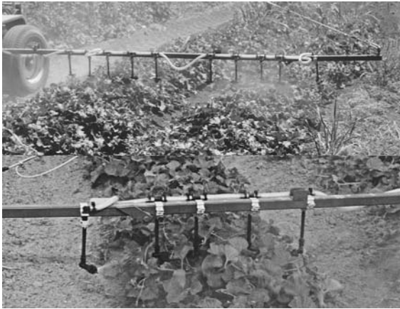
Fig. 1 Directed spray application of mycoinsecticide using conventional spray equipment that directs most of the spray into the cucurbit canopy. (Top) Spray designed to treat two rows of cucurbits. (Bottom) Close-up of drop tube and nozzle arrangement. Note height of nozzles in relation to plant canopy and rearward direction of spray
