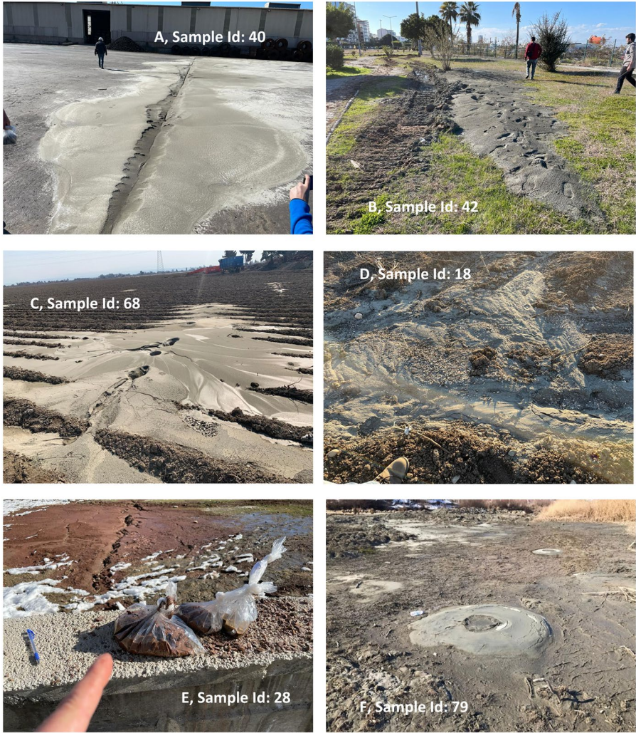
Fig. 7 A sample picture showing liquefied soil ejecta retrieved from six regions A through F
