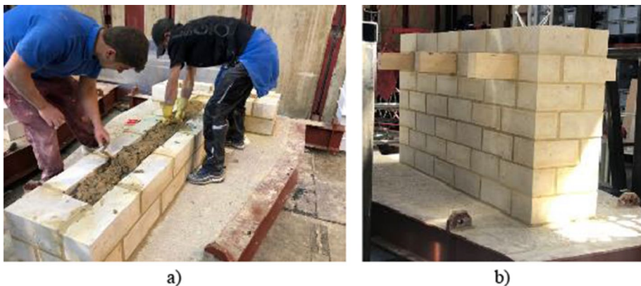
Fig. 7 Wall construction phases: a infilling between the outer leaves; b finished three-leaf wall
