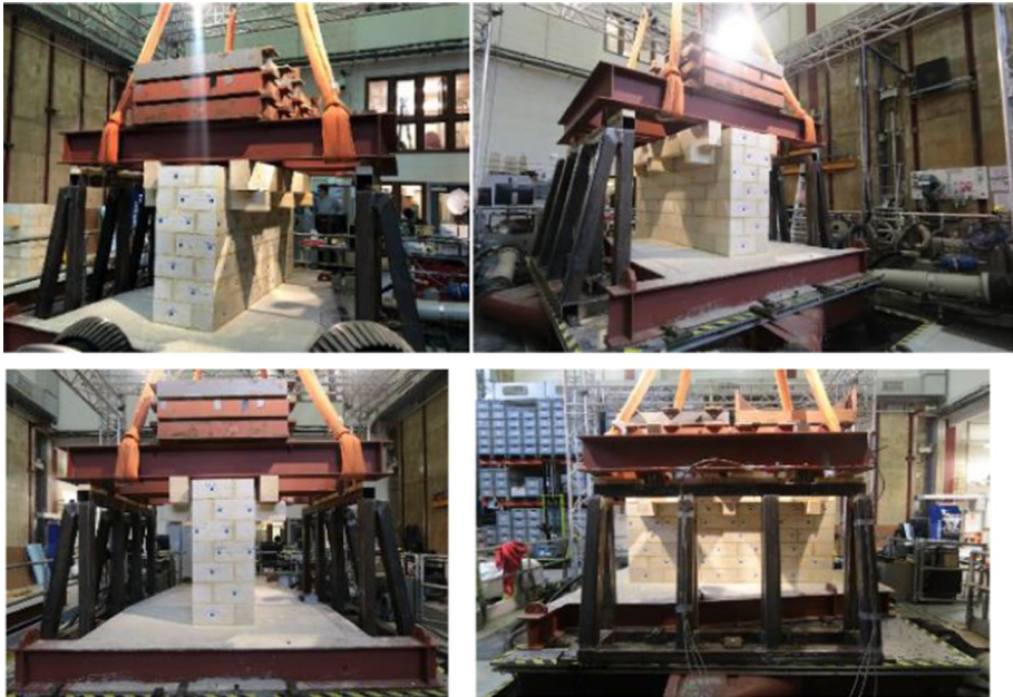
Fig. 9 Wall specimen before the test
