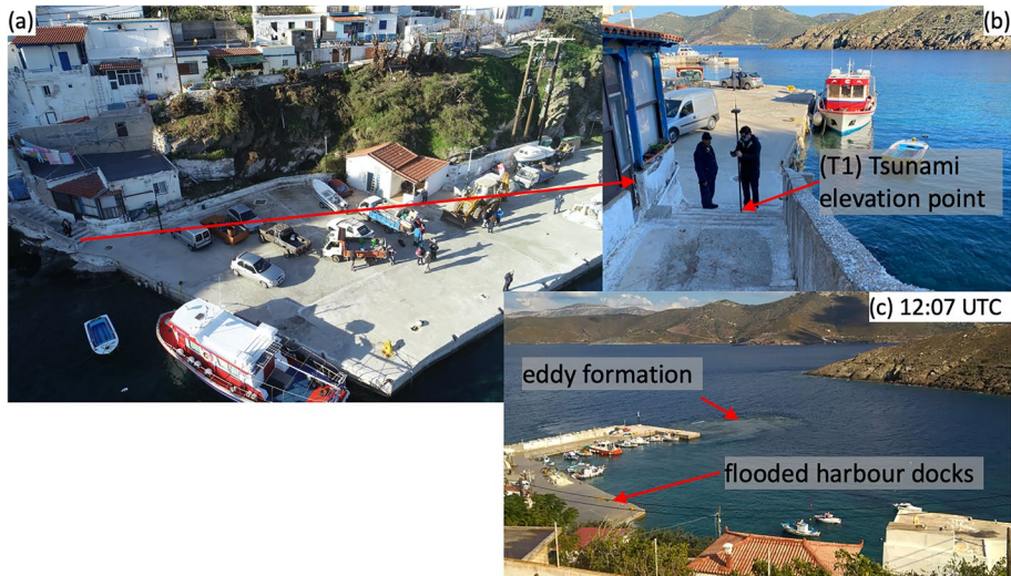
Fig. 8 a Aerial picture showing the harbour of Thimena, and the tsunami elevation data point measured on the first step of the staircase connecting the harbour to the town ( b ). c A frame from an eyewitness video showing an eddy forming at the corner of the harbour dock during the second drawdown phase and the harbour docks being already flooded
