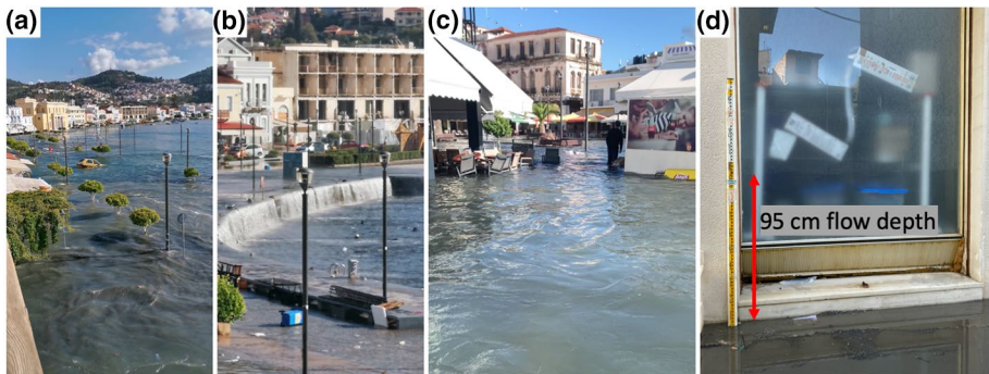
Fig. 13 a–c Eyewitness pictures from the second and largest flood in Vathi, Samos. d A characteristic flow depth point identified on a dusty shopping window the day after the tsunami along Tompazi St. in Vathi (data point S7–12)
