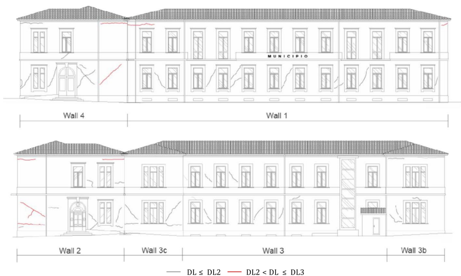
Fig. 8 Damage pattern in the Pizzoli town hall (according to the damage survey carried out by the ReLUIIS 2017–2018 Task 4.1 Workgroup on 26th June 2017). The walls numbering refers to that introduced in the Annex 1-Benchmark Structures Input Data
