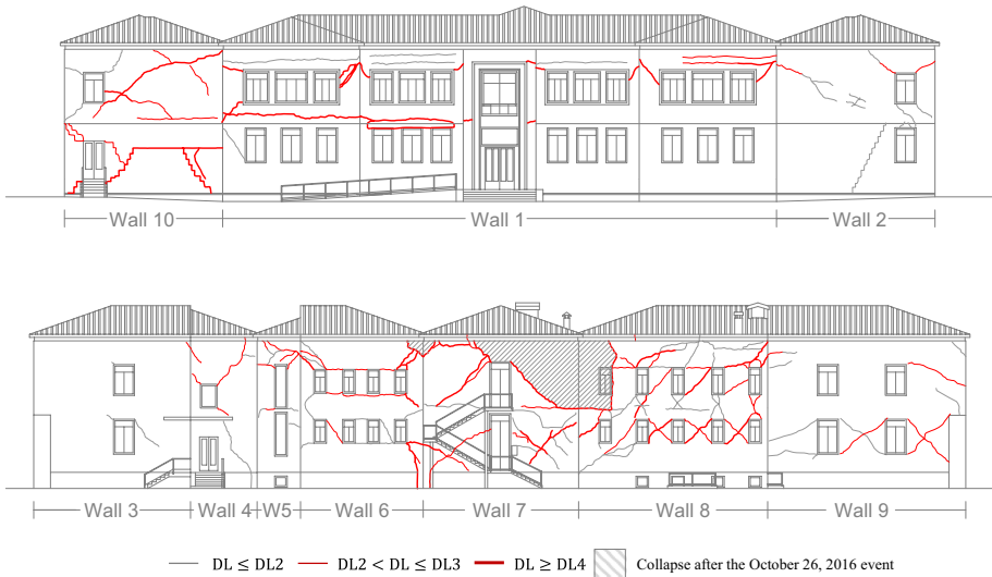
Fig. 7 Damage pattern in the P. Capuzi School according to the damage survey carried out by S. Cattari and D. Sivori on 8th December 2016. The walls numbering refers to that introduced in Annex I-Benchmark Structures Input Data
