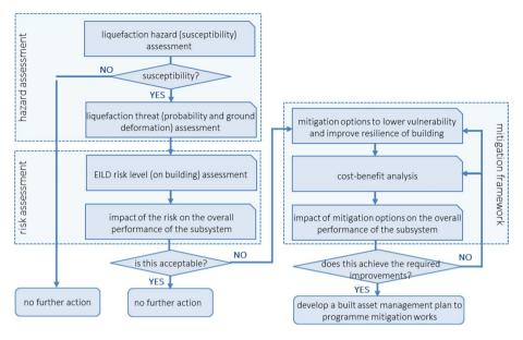
Fig. 6 The LIQUEFACT software flow diagram
